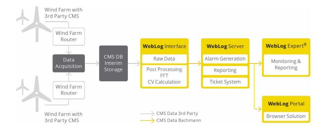
The data collected by the SKF CMS is sent to a monitor server via a router  $^{1)}$  in the wind farm, which forwards the data to a SKF database on a MSSQL server for temporary storage. From there, the WebLog Interface transfers the existing source
