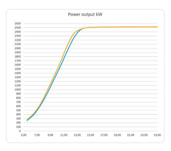
3% more yield: The intelligent control algorithms behind the retrofit solution take the current condition of rotor blades into account. This increases the tip speed ratio (TSR). The result: up to 3% increase in annual energy production.
